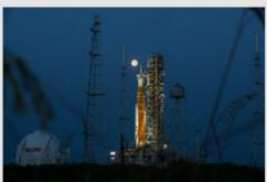
tall, ever developed by NASA. It will be used to send astronauts back to the Moon. It is also the most powerful rocket to launch since NASA's final Saturn V "Moon rocket" took the Skylab space station into Earth orbit in 1973. At 8.8 million pounds (3.9) million kg) of thrust, SLS is the most powerful rocket ever produced.
